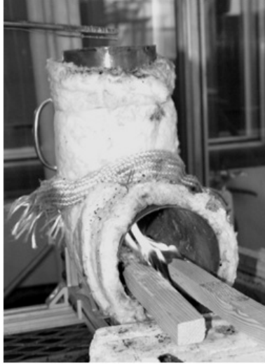
Figure 1: Insulated Rocket Elbow Stove.
