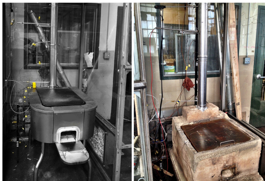
Fig. 2. The two stove models used in this work. Stove A (left) has been recently developed at the EECL for a commercial partner. Stove B (right) was constructed at the EECL based on design drawings for the “Justa” model provided by the Honduran government.
